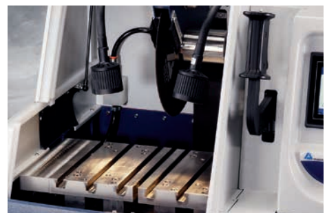
AbrasiMatic 300 standard machine without X-axis direction sectioning.
